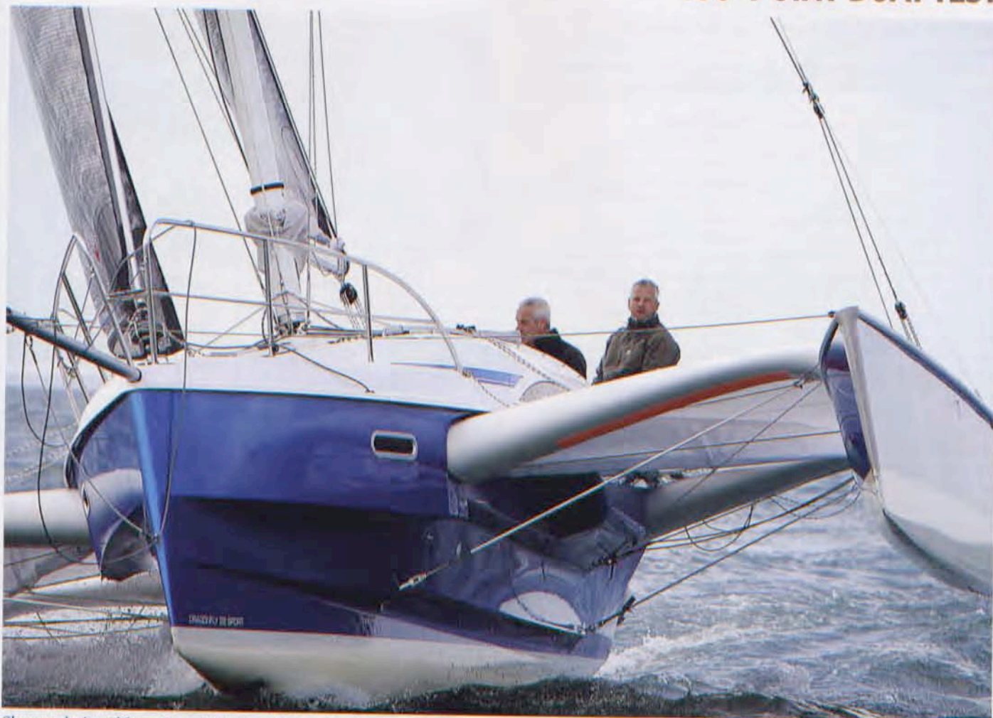
She was designed from the outside in, so the topsides have recesses to accommodate the stowed outriggers. The sprayrails also improve space below
