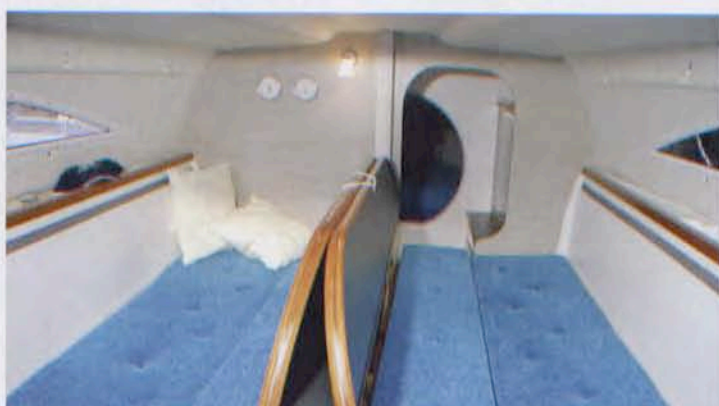
A clever rearrangement of the saloon leaves you with two good single seaberths, but they do restrict others moving fore and aft, so not ideal
